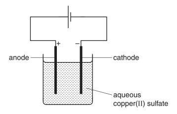
A solid is produced at the cathode. A gas is produced at the anode.
